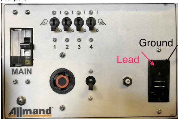
• If the GFCI and main breaker is any lower than 120/240 volts then check the capacitor in the generator end.
