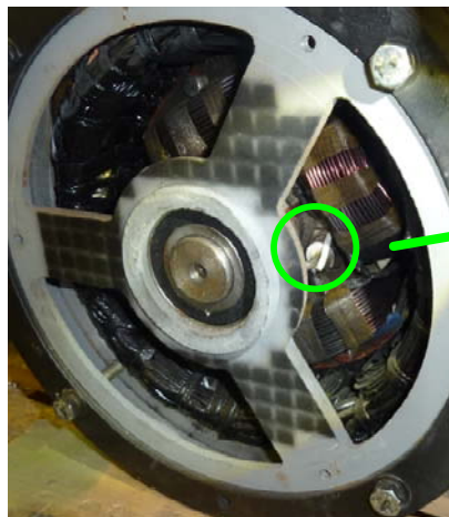
Figure 5 – Back of Unit with Diode Circled.
