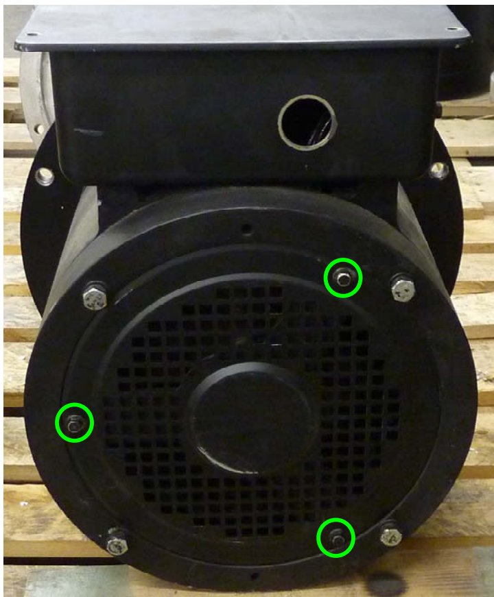
Figure 1 – Back of Unit with Cover. Use a 8mm or 5/16" socket to remove the three screws circled above.
