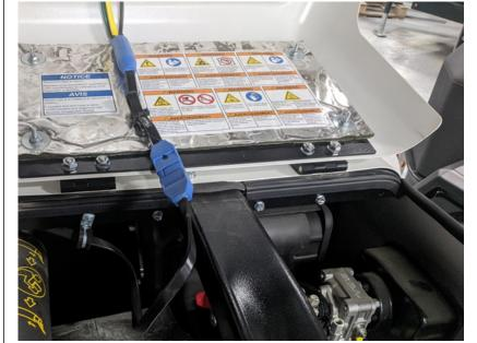
MEASURE APPROXIMATELY 10 1/2" OF WIRING FROM THE ROOF PANEL ZIPTIE. INSTALL THE LOWER HARNESS BEHIND THE CANISTER AND ZIP TIE THE CONNECTOR TO THE OUTSIDE HOLE OF THE DOOR HINGE. MOVE THE CUSH CLAMP TO THE BOLT LOCATION IN THE ROOF PANEL AS SHOWN. THIS SHOULD PROVIDE ENOUGH CLEARANCE FOR THE TAIL LIGHT HARNESS AND PLUGS TO REMAIN FAR AWAY FROM ANY HEAT SOURCES INSIDE THE COMPARTMENT. THE FINAL RESULT IS SHOWN BELOW.
