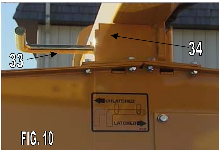
FIG. 10 REAR TOWER SUPPORT
