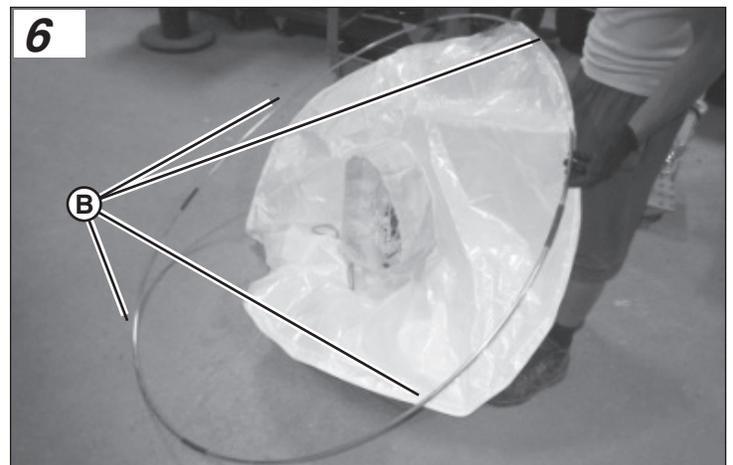
6. Position the balloon shade over the extension rod on top of the light cage, with the cuffed opening of the shade facing toward the light cage. See Figure 8. Secure the top of the balloon shade to the extension rod with the supplied wing nut (F, Figure 7). Tighten securely.
