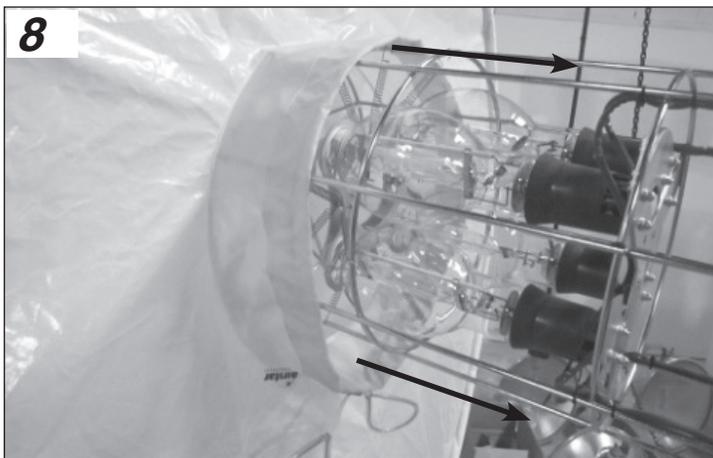
8. Pull the loop handles of the securing cable against the locking clamp to tighten the cuff against the underside of the light cage bottom. See Figure 9.
