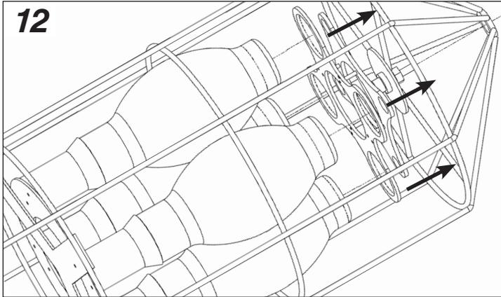
4. Carefully position the bulb holder over the top of the bulbs, using the springs (not shown) to secure the holder in place. See Figure 13.
