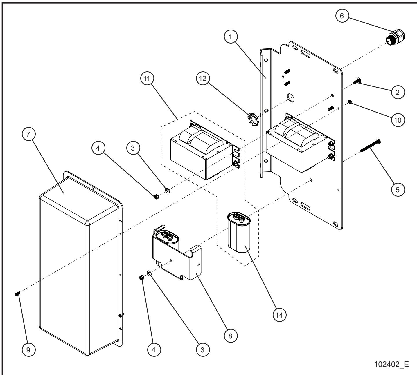
**5.8 - 1000W 50Hz 120V Ballast Box Assembly**SN 07-000001 and UP
