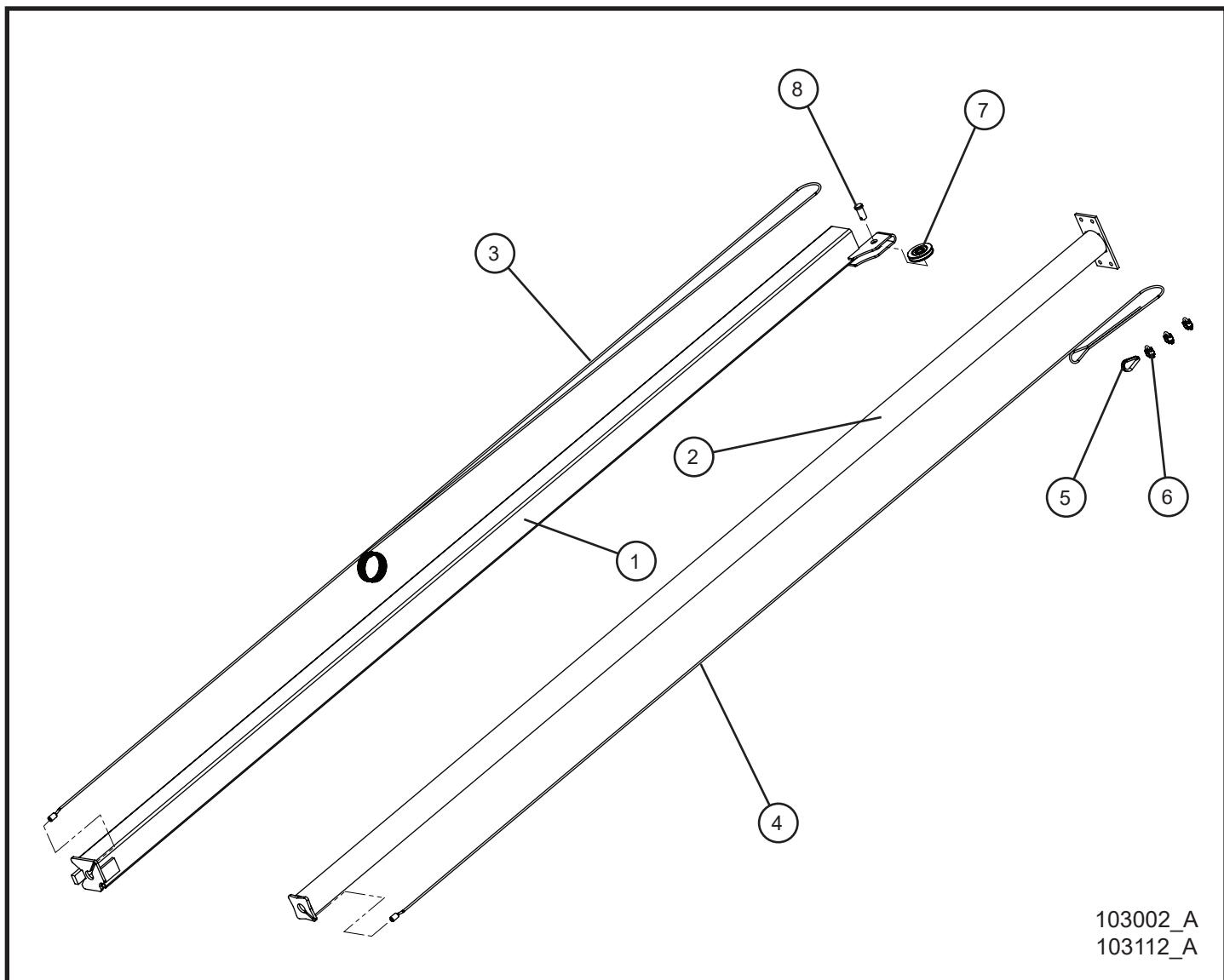
**3.3 - Laydown Tower Parts New Style (2 of 2)**
