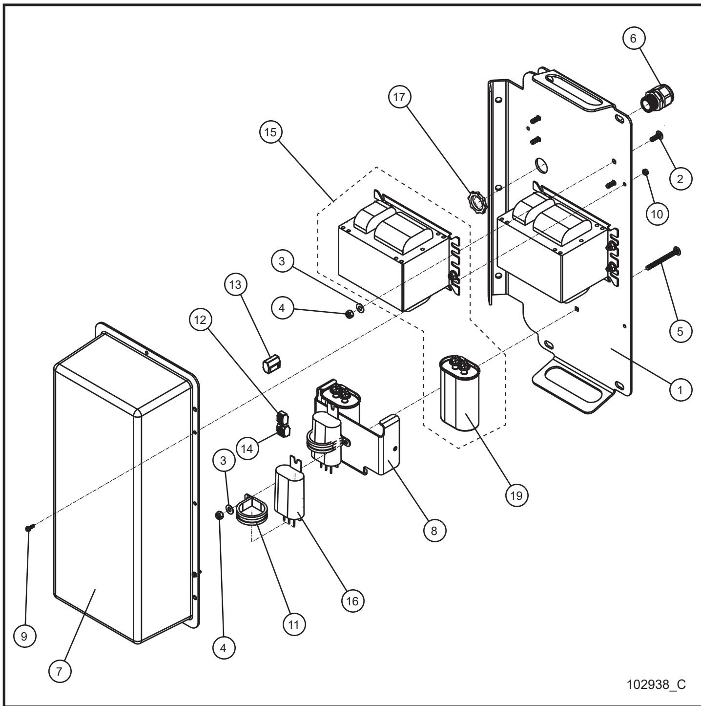
**5.2 - 1000W HPS 60Hz 120V Ballast Box Assembly**SN 07-000001 and UP
