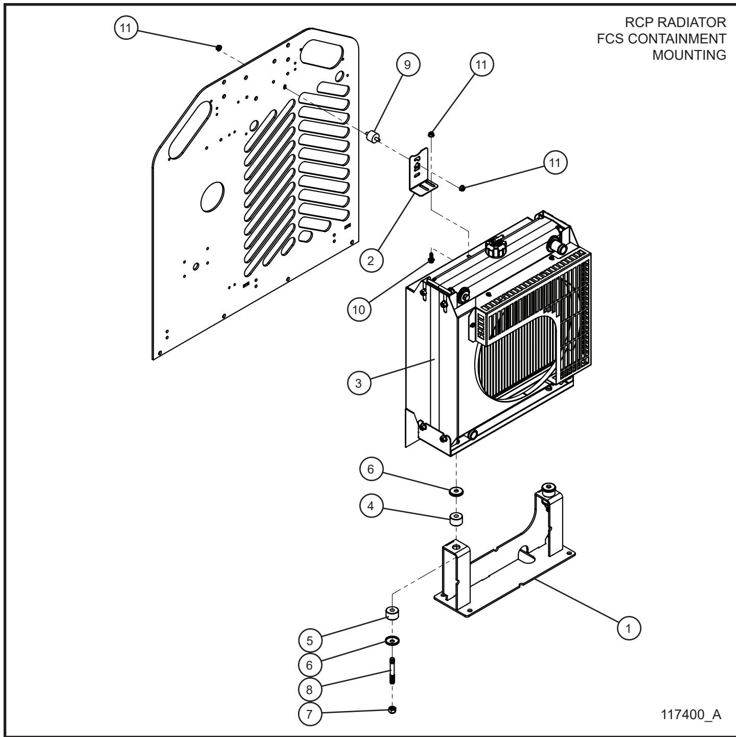
**9.4 - CAT/Perkins 1.1 Engine (Fan-to-Fly) Assembly Group (6 of 7)**SN 07-000001 and UP
