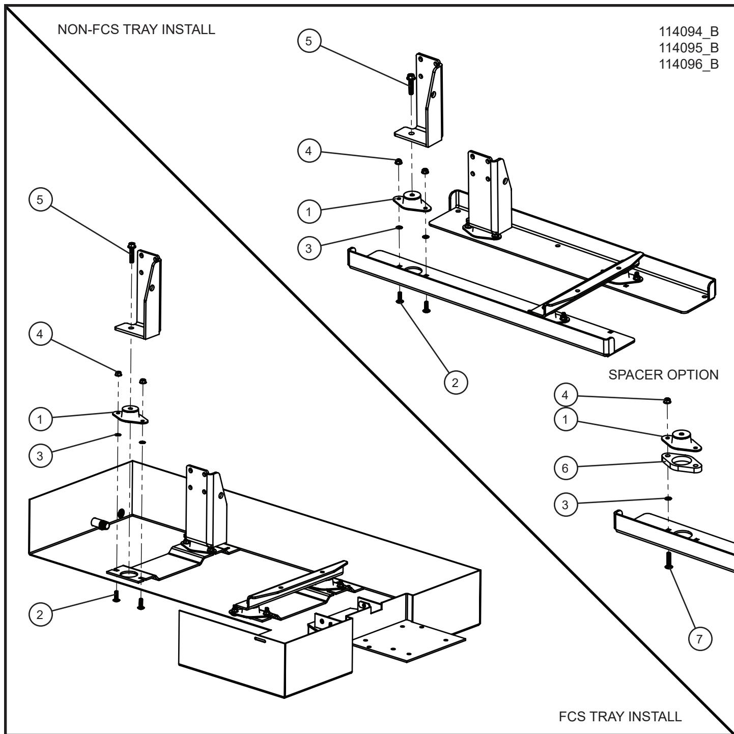
**8.13 - Engine Isolator Threaded Mounts**SN 07-000001 and UP
