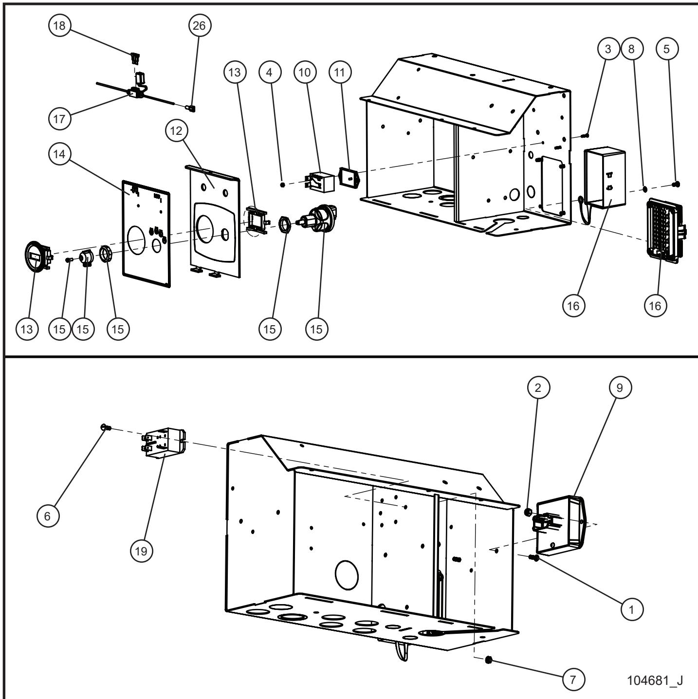
**6.25 - SLS Key Start Engine Control I (with Timer Relay)**SN 07-000001 and UP
