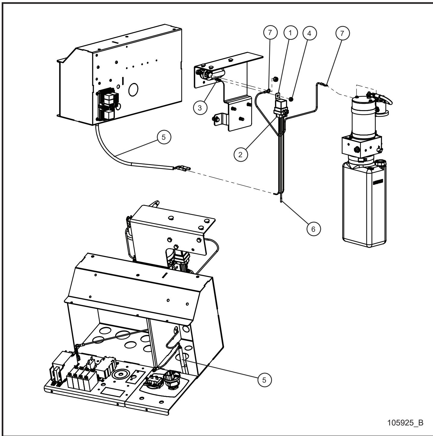
**4.11 - Vertical Tower Pump-Key Switch Relay**
