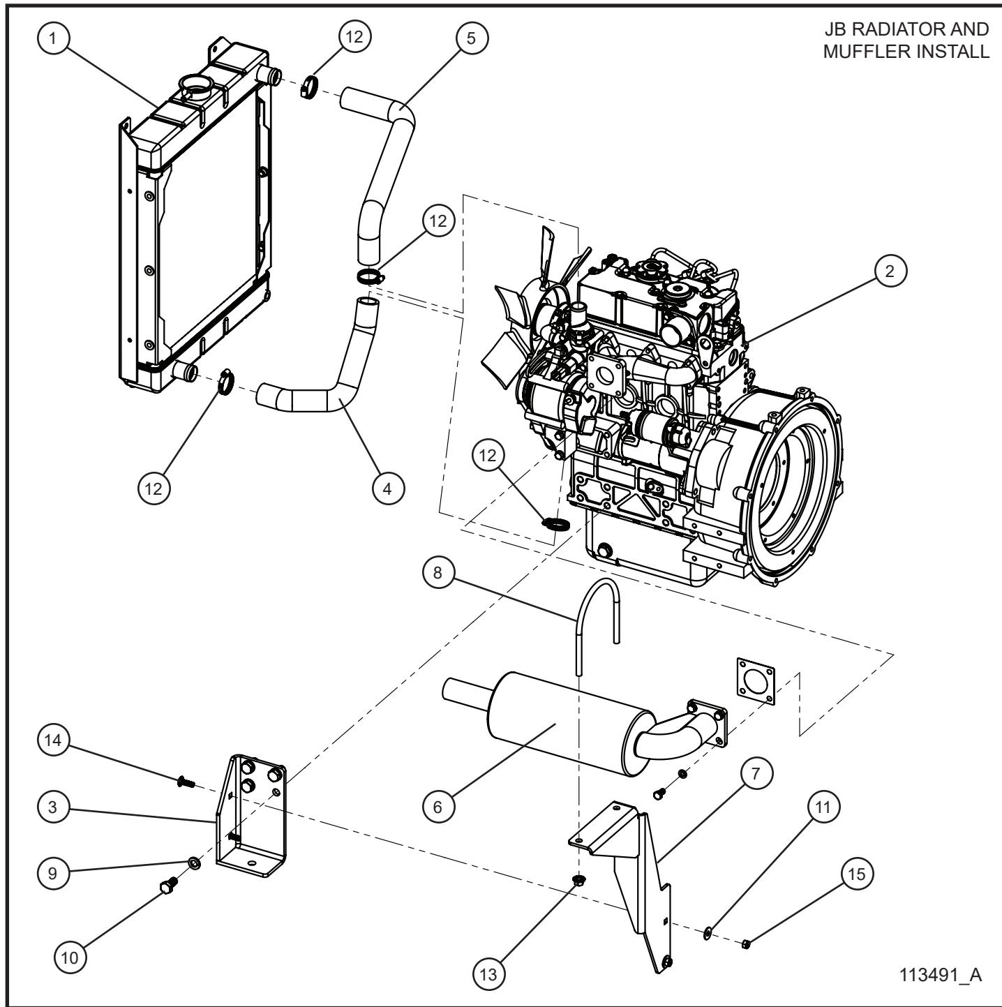
**9.4 - CAT/Perkins 1.1 Engine (Fan-to-Fly) Assembly Group (1 of 7)**SN 07-000001 and UP
