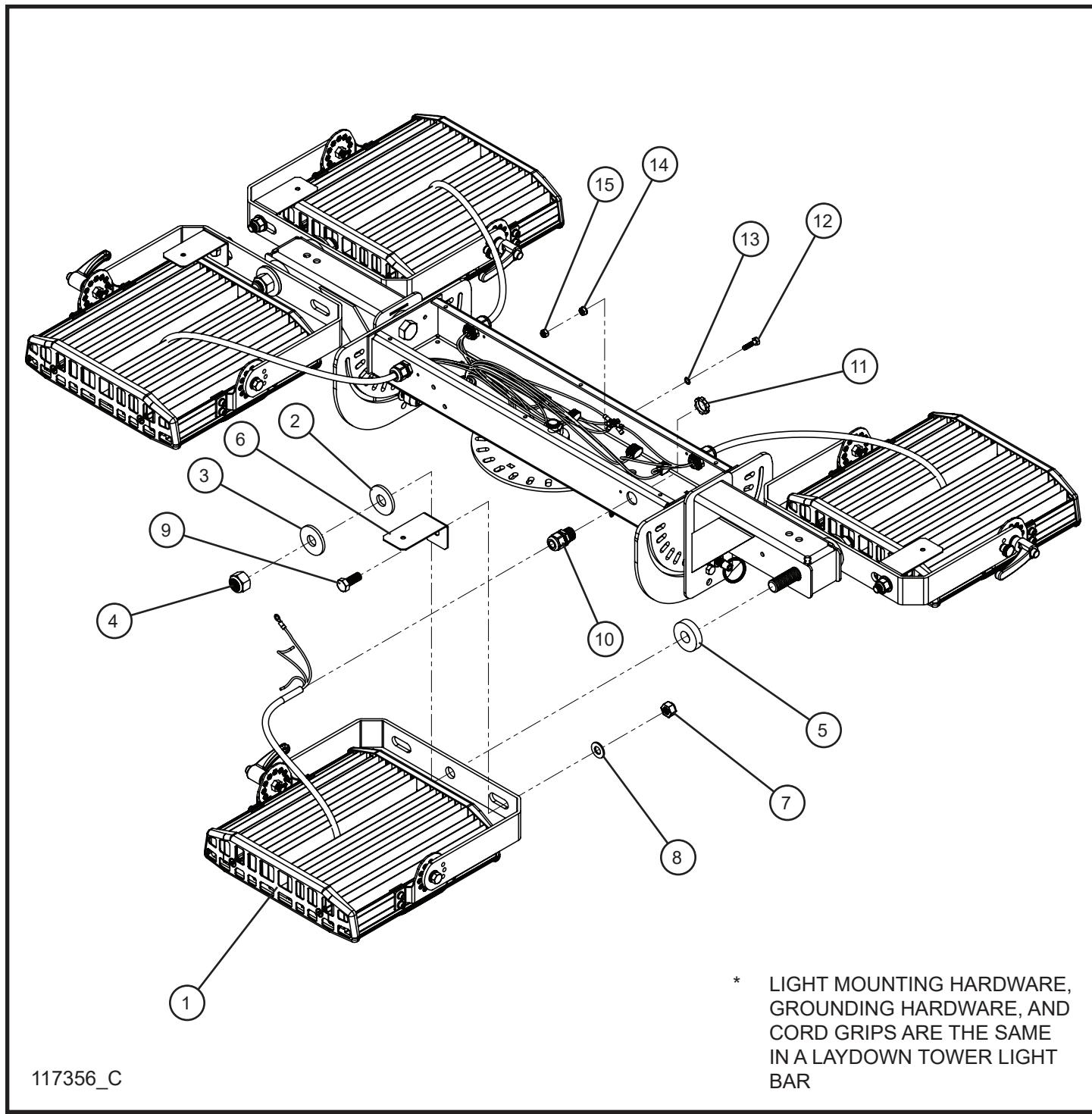
**5.17 - Conssin COB LED Lamp Install Group**SN 07-000001 and UP
