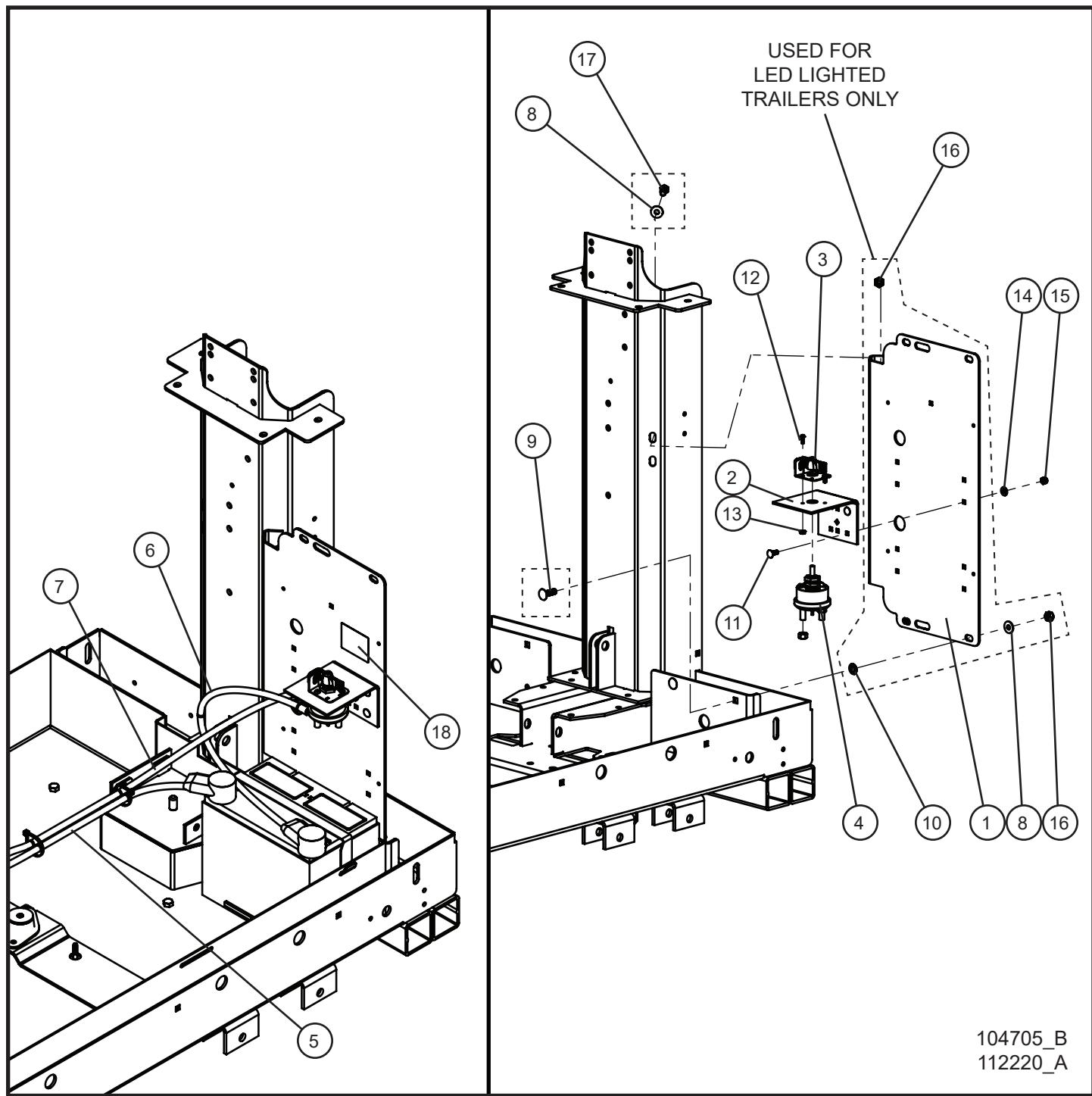
**8.3 - Battery Negative Pole Disconnect**SN 07-000001 and UP
