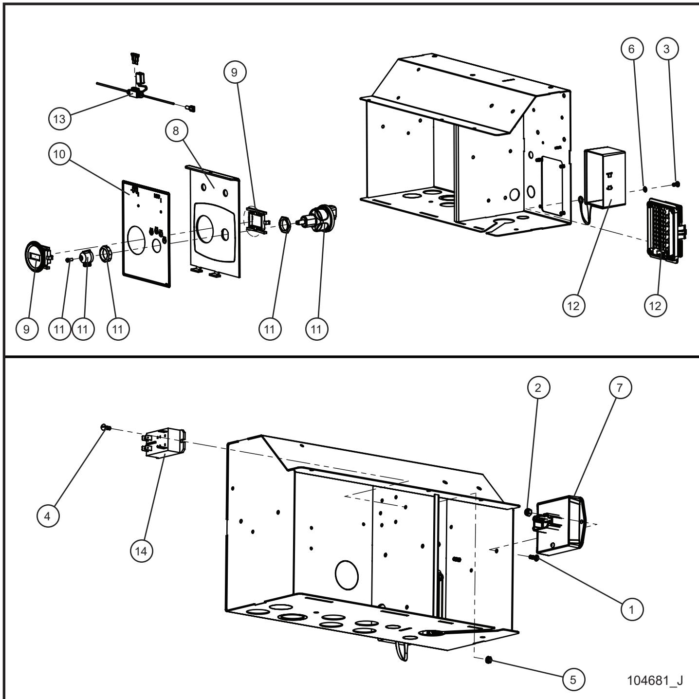
**6.27 - SLS Key Start Engine Control II (no Timer Relay)**SN 07-000001 and UP
