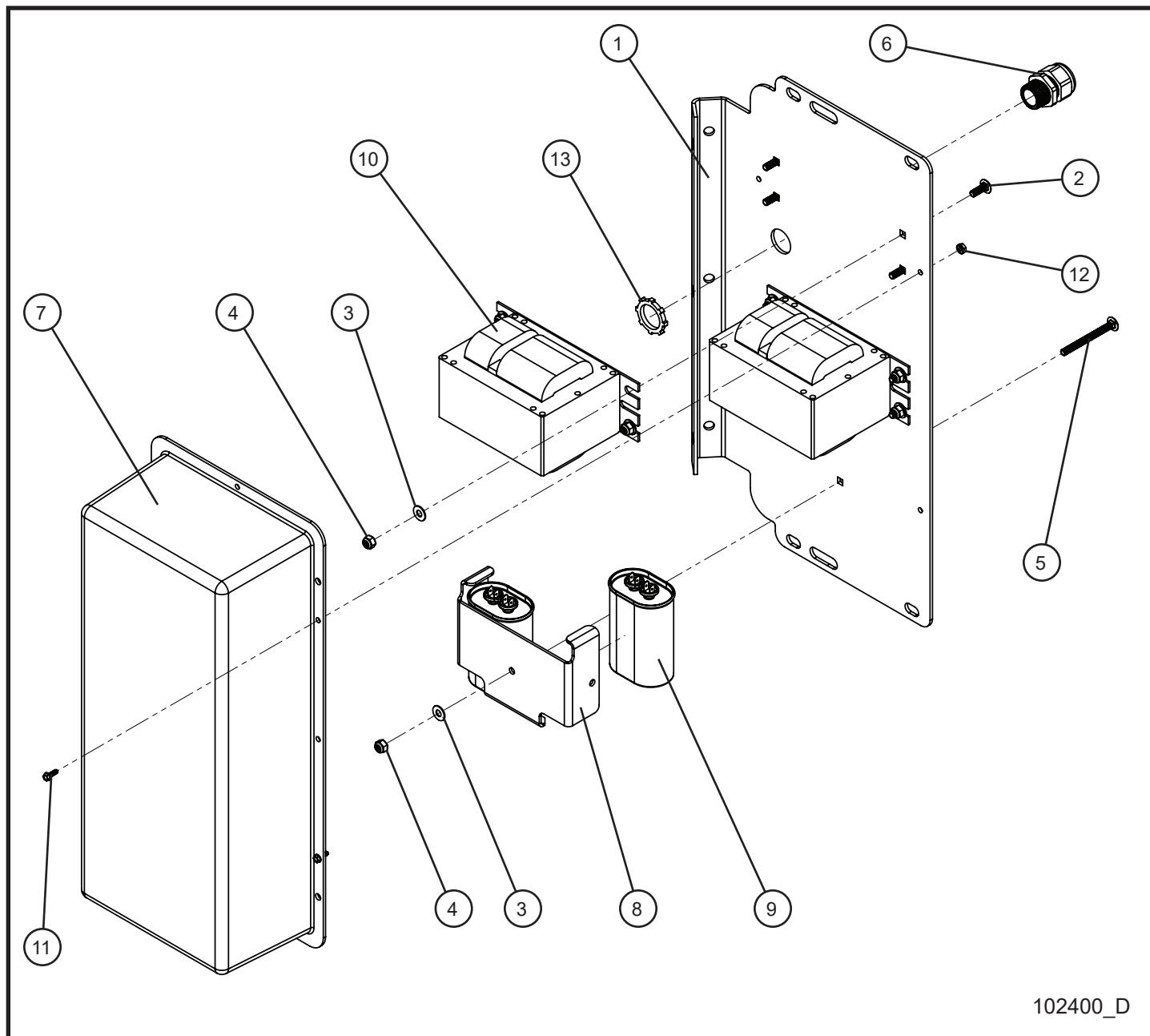
**5.6 - 1000W 60Hz 120V Ballast Box Assembly**SN 07-000001 and UP
