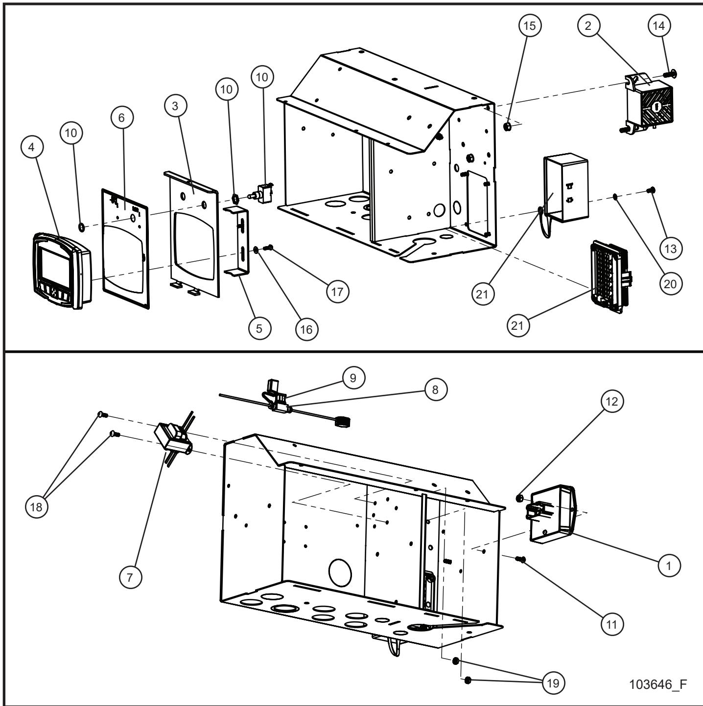
**6.29 - LSC Start Engine Control with Toggle Switch**SN 07-000001 to 07-000142
