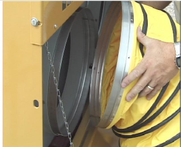
Duct ready for installation on heater using 16" Slip-Lock Connectors (pn 848974)
