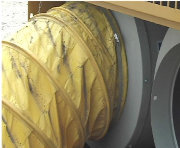
16" screw clamp (pn848176) used here to attach duct (pn848172)
