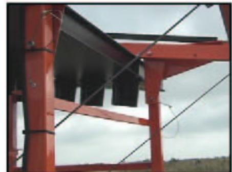
The trailer should be properly set up with the jack stabilizers, sand bags, etc. in position before leaving the **ALLMAND ECLIPSE 2220/SE SERIES** deployed in the traffic control area. Periodically inspect the tongue, pins, safety chains, hitch, all nuts, bolts, cable clamps, wiring, etc. for wear and repair or replace if necessary.
