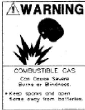
PART NO. 090159 Location: Above battery on tower support inside enclosure.
