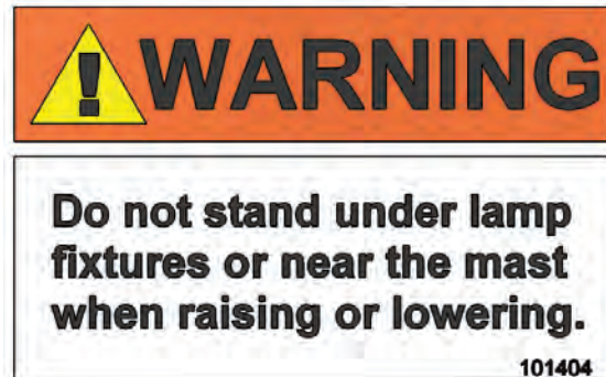
PART NO. 101404 Location: On either side of mast assembly immediately above roof panel .
