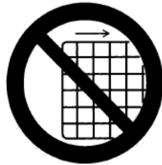
090400 DO NOT OPERATE WITH GUARD REMOVED
