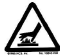
090417 BURN HAZARD HOT SURFACE
