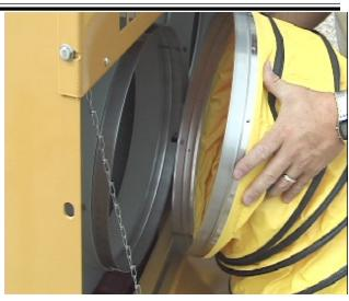
Duct ready for installation on heater using 16" Slip-Lock Connectors (pn 848974)
