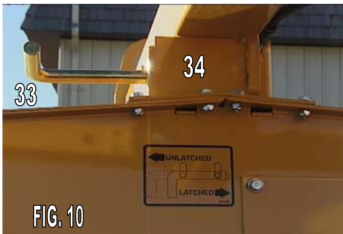
FIG. 10 REAR TOWER SUPPORT
