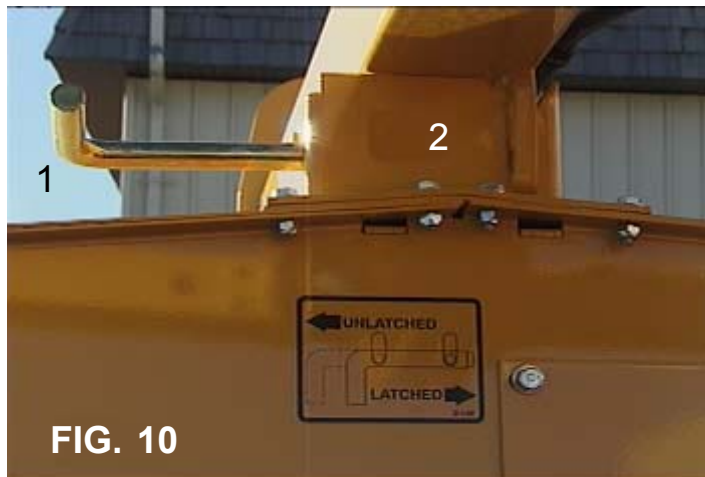
FIG. 10 REAR TOWER SUPPORT
