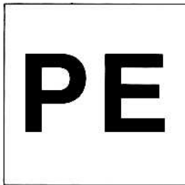
DD-416 PROTECTIVE EARTH GROUND
