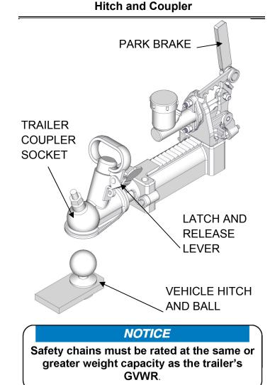
The trailer's safety chains prevent the trailer from completely detaching from the vehicle when underway. In the event the trailer separates from the vehicles hitch and ball.
