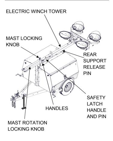
Before raising the light tower, visually inspect the equipment for worn or damaged parts and replace as necessary.
