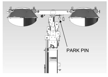
With the light bar park pin released, the light bar is designed to be manually rotated with enough resistance so that the bar will stay in the desired position once the operator has directed the lights on the work zone.
