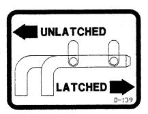
PART NO. D-139 Location: On rear panel under the rear tower support.
