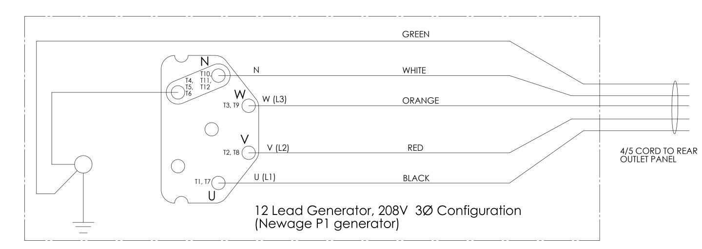
12A 208 Volt 3 Phase 4 Light Manual Winch Ballast Panel Wiring Diagram
