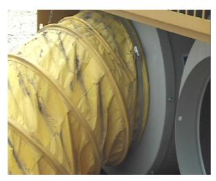
16" screw clamp (pn848176) used here to attach duct (pn848172)
